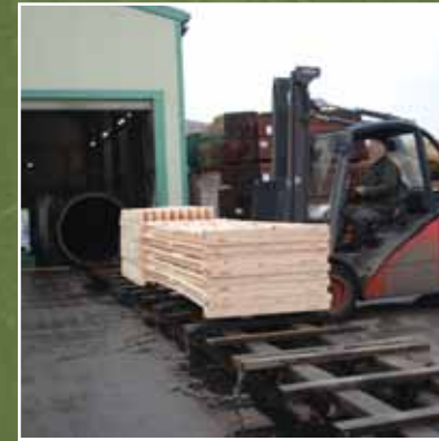
Pressure treatment of timber is carried out on site at Linnell Bros.
